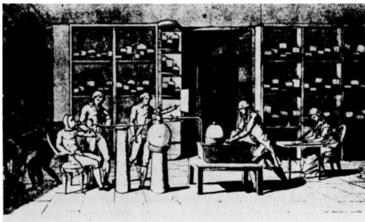
FIGURE 2 Lavoisier in his laboratory during his studies on respiration (from a sketch made by Madame Lavoisier.) This brilliant chemist measured the volumes of air breathed by a man at rest and at work and showed that his temperature remained constant. He concluded "respiration is merely a slow combustion of carbon and hydrogen which is similar in every respect to that which occurs in a lighted lamp or candle...."
