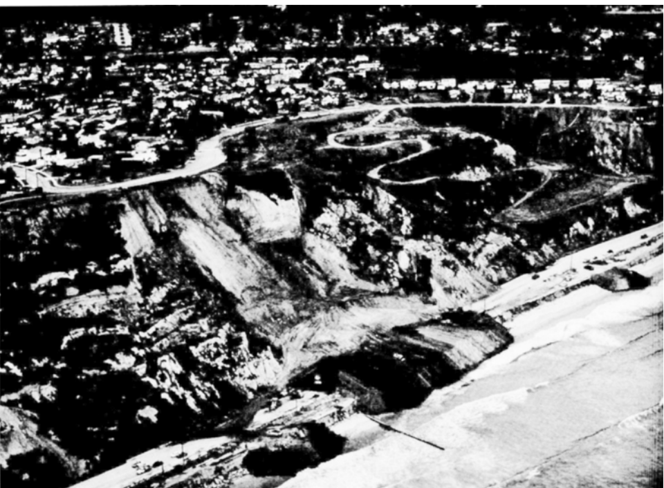
FIGURE 4A A seacliff landslide at Pacific Palisades, California. Sudden failure of weak, water-saturated sedimentary rocks sent a large tongue of debris across the coastal highway, which was being cleared when this photograph was taken in 1958. Remnants of older landslide masses can be seen along adjacent parts of the steep, seaward-facing slope, which has been slowly encroaching upon the settled area in background.
