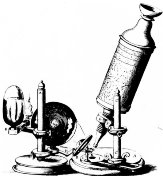
FIGURE 2 This engraving, cut by the eminent British scientist and philosopher Robert Hooke, was published in 1665 in the first treatise devoted solely to microscopy. It shows Hooke's improved compound microscope with its hemispherical lens objective and plano-convex lens eyepiece. A spherical condenser concentrated rays from a lamp on the specimen.
