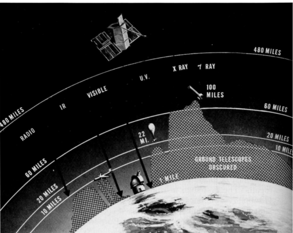
FIGURE 3 This shows the way in which the Orbiting Astronomical Observatory has expanded the spectra available for astronomy. (IR = infrared; U.V. = ultraviolet)
