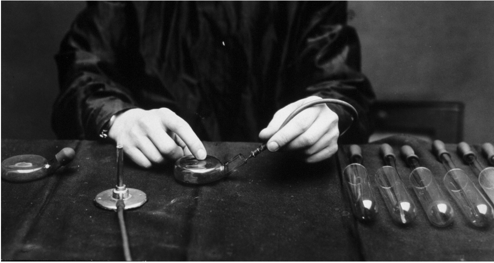
Figure 4. This undated photograph shows the hands of a technician manipulating the specially designed “Carrel flask” and the aspiration device Carrel designed in the 1920s and widely used into the 1950s. Alexis Carrel Papers, Rockefeller Archive Center.
